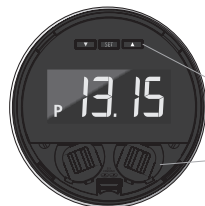
Under the front cover Keys for setting (See page 18 to 20 for details). Battery compartment
